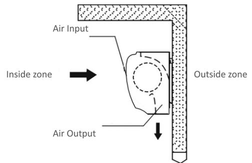
**3.3** The maximum mounting hight from the floor is 2,3 metres. In case the door opening width is bigger than the length of the device, the two or more units should be installed in series with the breaks of 20-40 mm between them.
