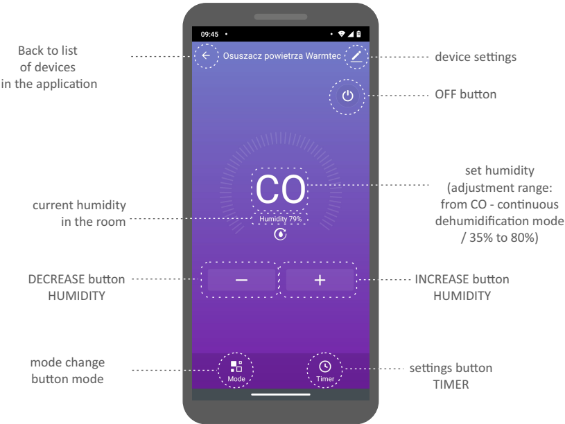
control interface - device switched on (dehumidification mode + circulation)
